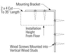
• Secure the bracket with wood block to the back wall so that it is 84" (or your installation height) from the finished floor. See illustration.
